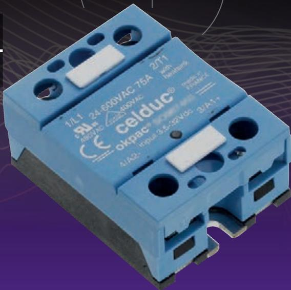
With our integrated back to back thyristors technology (direct copper bonded ceramic) offering a very high life expectancy, our SSRs are perfectly adapted to the requirements of medical equipment manufacturers. We offer a wide range with thyristor ratings up to 125A / 660V as well as a wide AC-DC input range with regulated current models. Removable flaps for IP20 protection.
