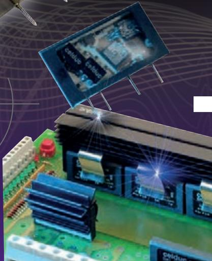
celduc offers an extensive range of PCB solid state relays suited to applications that demand long life and high reliability and where fast response and high switching rates are required. AC versions are available from 5A up to 75A thyristor rating.
