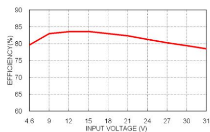
SSR01-12S05 Efficiency VS Input Voltage
